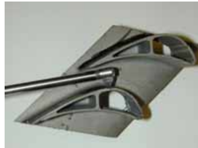
Model: AE12205 Frequency: 12 MHz Height: 0.350" Removable delay line
