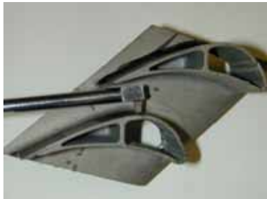
Model: PTX2 Frequency: 15 MHz Height: 0.350" Removable delay line
