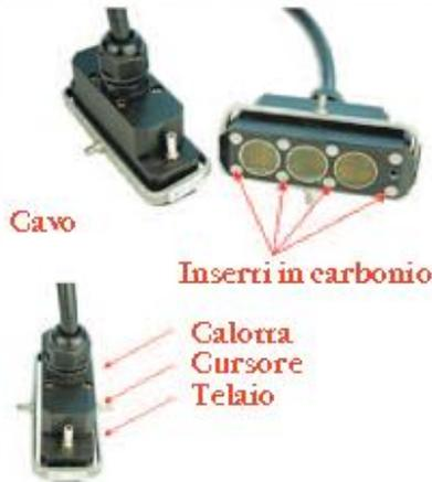
The flaw detector comprises two probe units:
